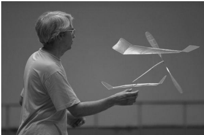
THE CHAMPION'S MODEL, DIDIER, LIFTING OFF. THE FUSELAGE AND THE WINGS ARE TWISTED BY RUBBER TENSION. IT IS CLEAR THAT HE IS CLOSE TO THE LIMITS OF HIS MODEL
