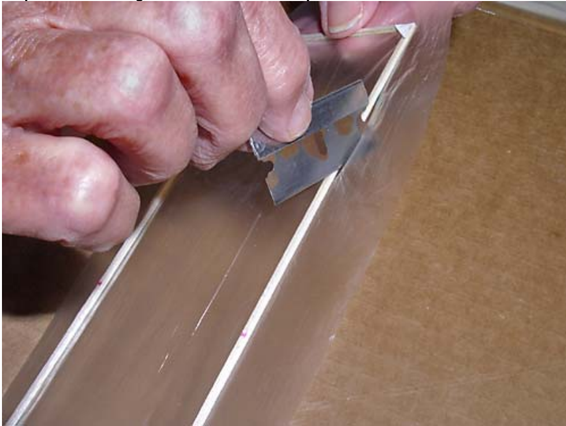
Cutting the wing and stabilizer from the plastic
