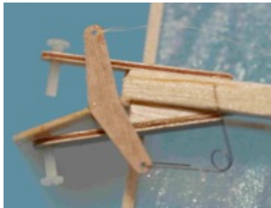
Ray Harlan's auto-rudder viewed from the bottom. Adjustment screws are 090. The line attached to the rudder horn goes to the swinging pendulum on the tow hook.
