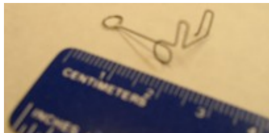
Close-up of the spring action ring, made from 0.014" music wire.
