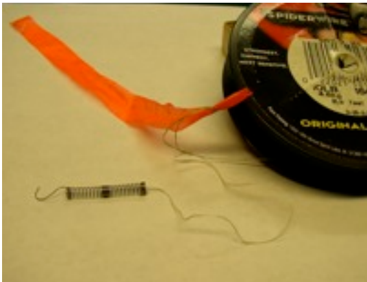
Towline with a spring attached, one end forming a hook, for a stationary tow ring on the airplane.
